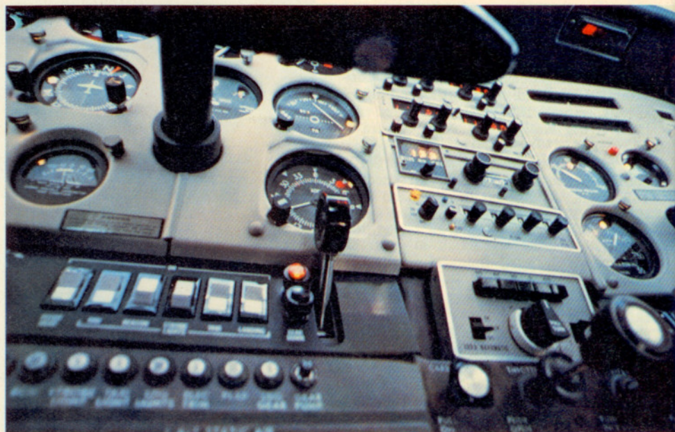
The gear handle is found just in front of the pilot's control yoke, and is adjoined by single up and down indicator lights.
