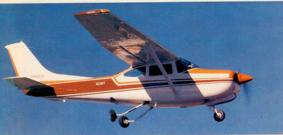
Up front, the new retractable Skylane houses a carbureted Lycoming 235-hp engine.
